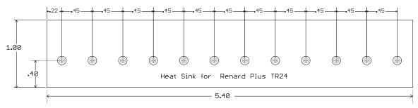
All measurements are in inches and all mounting holes are .150
